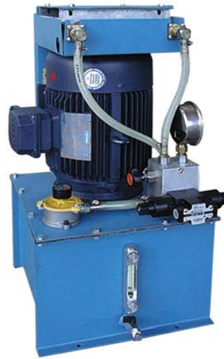
VTC5-7.5HPC3-G5 Vertical Tank: 1 station VTE-D03-1R manifold with integral relief valve and HE90 return line cooler
